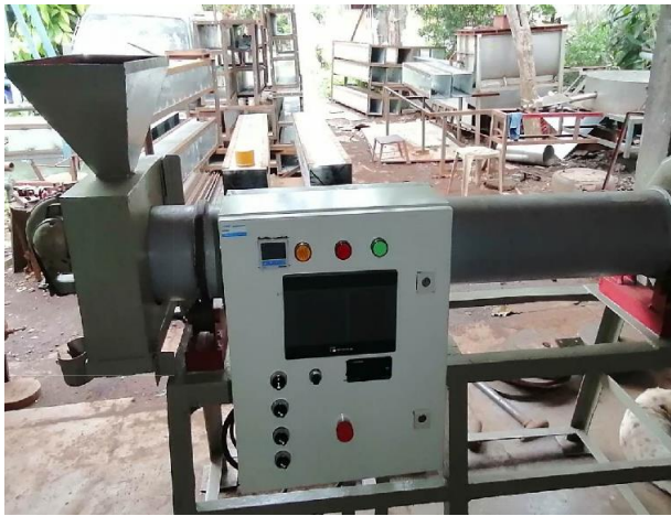
Figure 7. Control Panel Board
